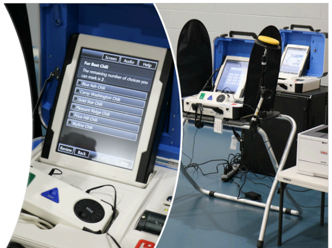
A picture of an Access Writer, an electronic ballot marking system with a touchscreen
